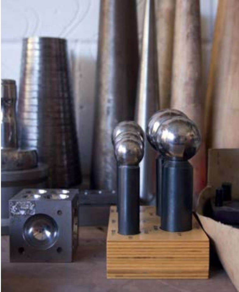
ABOVE A doming block and punches used for creating dome shapes, such as spoons, from flat sheets of metal. In the background are forming shapes made from steel and wood used to create cone shapes RIGHT Shona's jewellery bench in her studio at Cockpit Arts, Deptford
